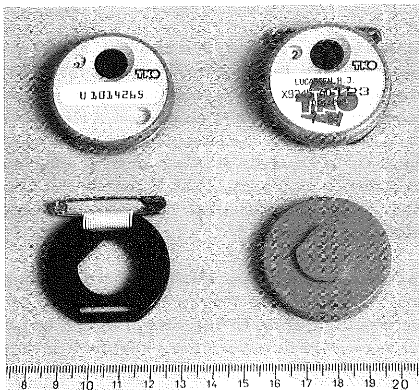
Fig. 3. The TNO TLD dosemeter, with and without the wearer's lable, showing the individual's name, number and issuing period
