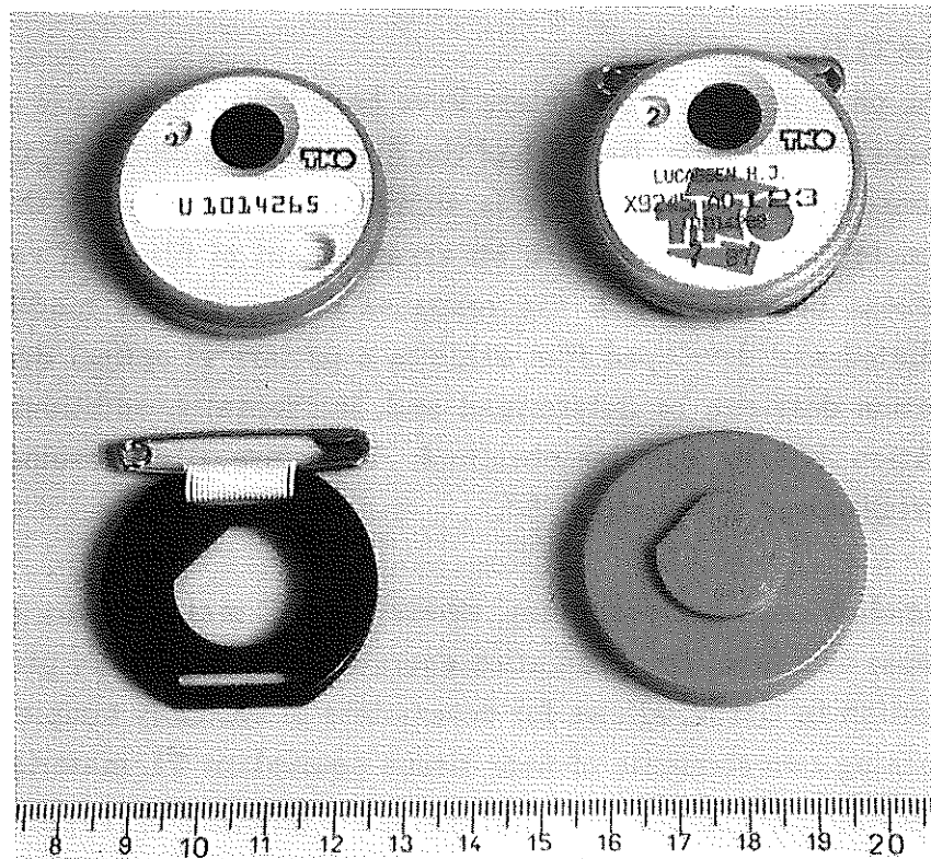
Fig. 3. The TNO TLD dosemeter, with and without the wearer's label, showing the individual's name, number and issuing period
