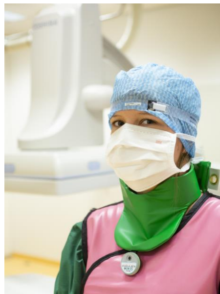
Figure 6-11 Illustration of the use of an eye lens dosimeter near the most exposed eye in interventional radiology.
