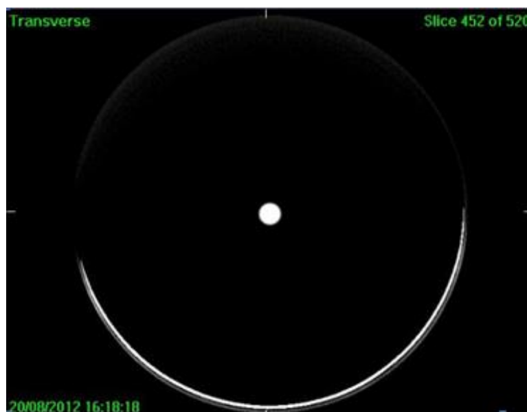
Figure 5.11. Transversal view of the halo artefact. Note that the white sphere in the middle is a ball-bearing phantom.
